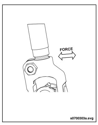
Fig. PM-10: Steering Driveshaft End Yoke Inspection
